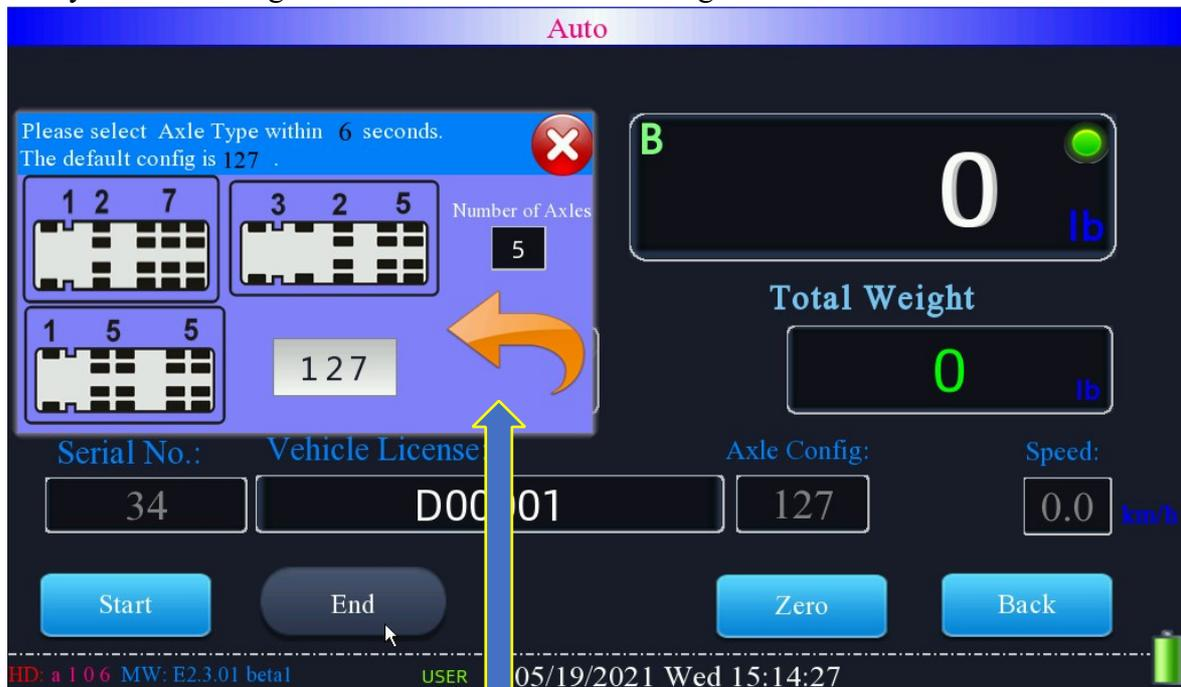
When axle numbers match more **Axle Type**, a window will pop up an showing all types of axles. A recommended type has been filled in, but operator could select different axle type according to reality case.
