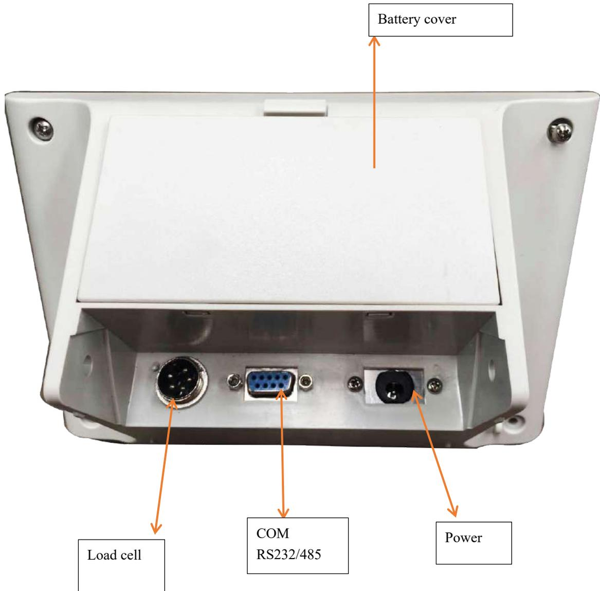
(figure 3-1-2 ) Function diagram of back view
