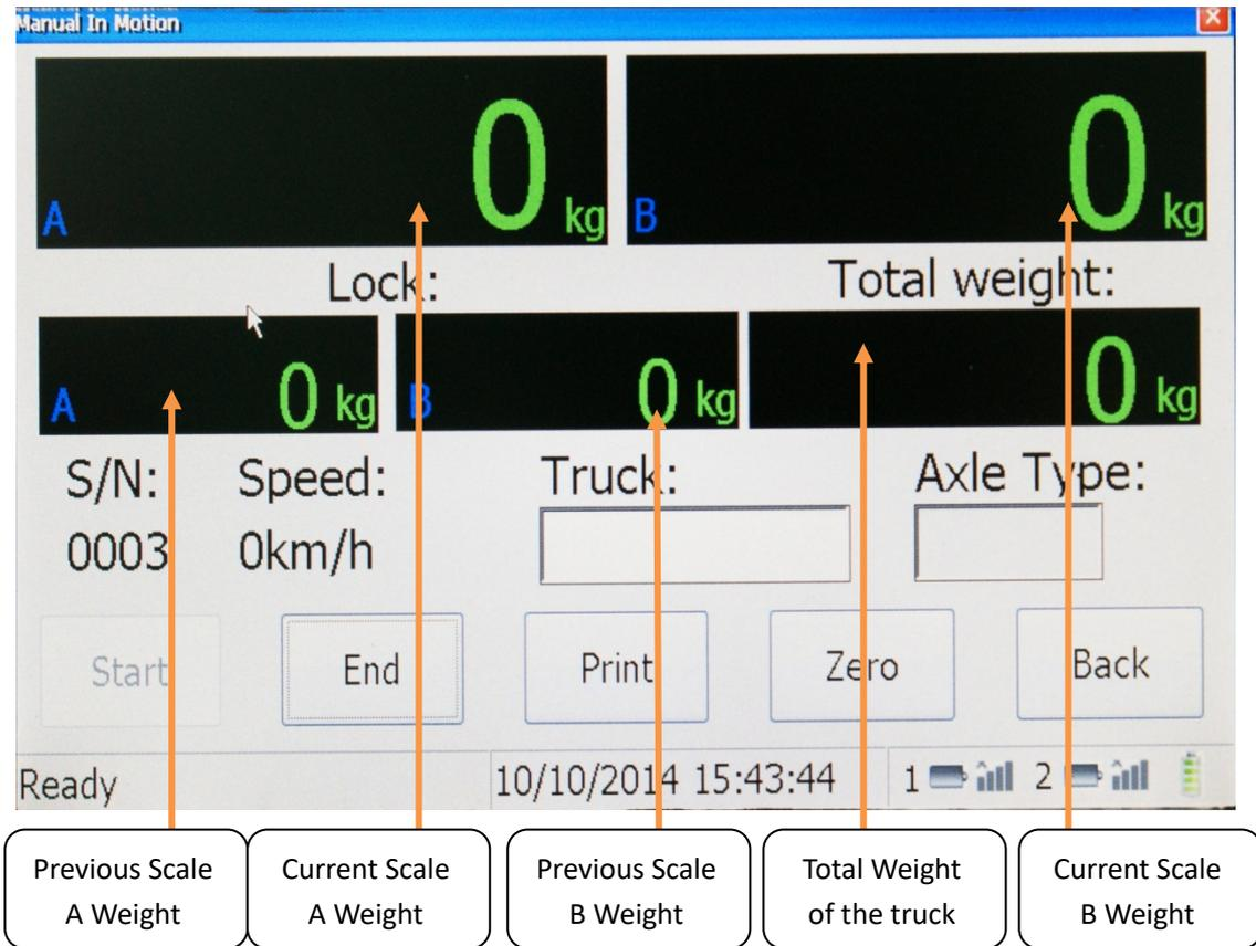
In **Manual** weighing mode, the "Axle Type" inputting is required and it is valid.
