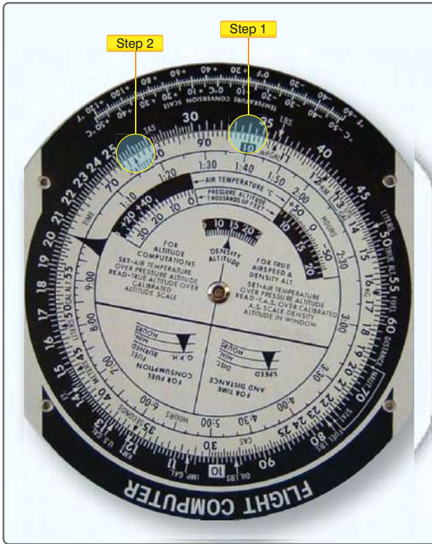
Figure 10-3. E6-B computer set up to multiply 340 by 78.
