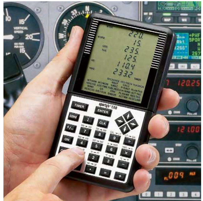
Figure 10-5. Dedicated electronic flight computers are programmed to solve weight and balance problems, as well as flight problems.
